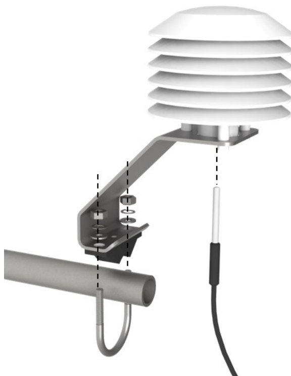
FIGURE 6-4. Mounting the IRGASON temperature probe
